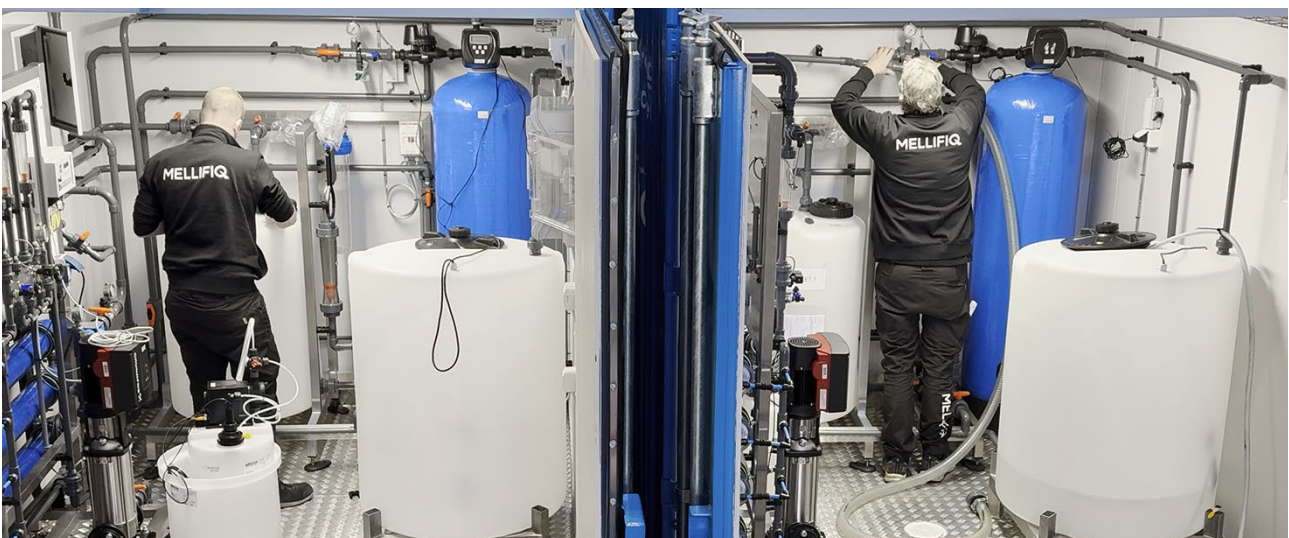
Final mounting and FAT of Water Maid CoraLuxe AC2-N systems for groundwater purification.
