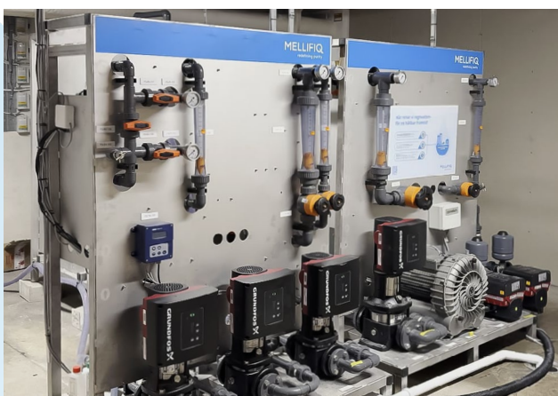
The stations are equipped with a cartridge filter, fan, permeate pump, backwash pump, and electronic meters for flow, turbidity, and temperature.
