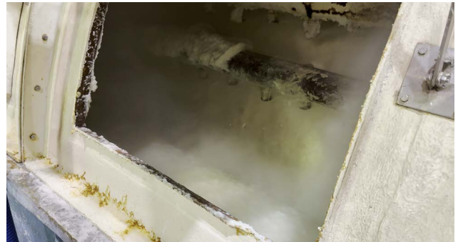
Washwater from the bleaching constitutes a large part of the effluent.
